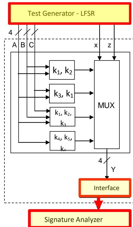
**2. Design of the experimental bench.** Use three different interface versions for experiments: 1 bit, 2-bit and 4- or more bit interfaces for respective n-bit Signature Analyzers
