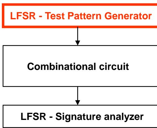
7. Generate test patterns by the BILBO tool for 10 different **polynomials**, and find the best structure for the LFSR
