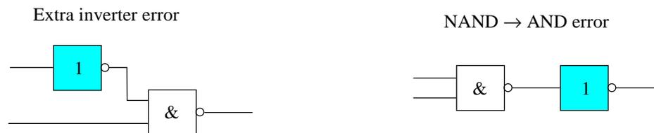
Fig. 4.3 Extra inverter and gate replacement errors
